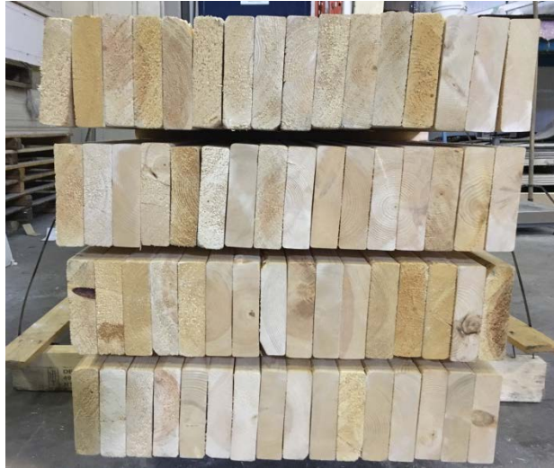
Figure 14. NLT surface profile (A)
