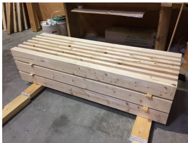
Figure 7. Constructed C panels
