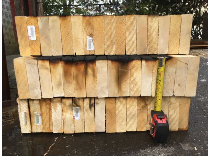
Figure 15. Depth of charring (A)
