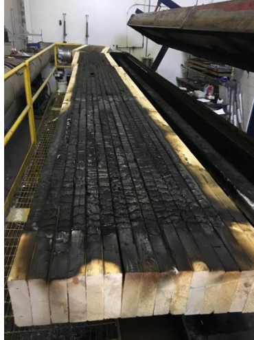
b) Exposed side after test
