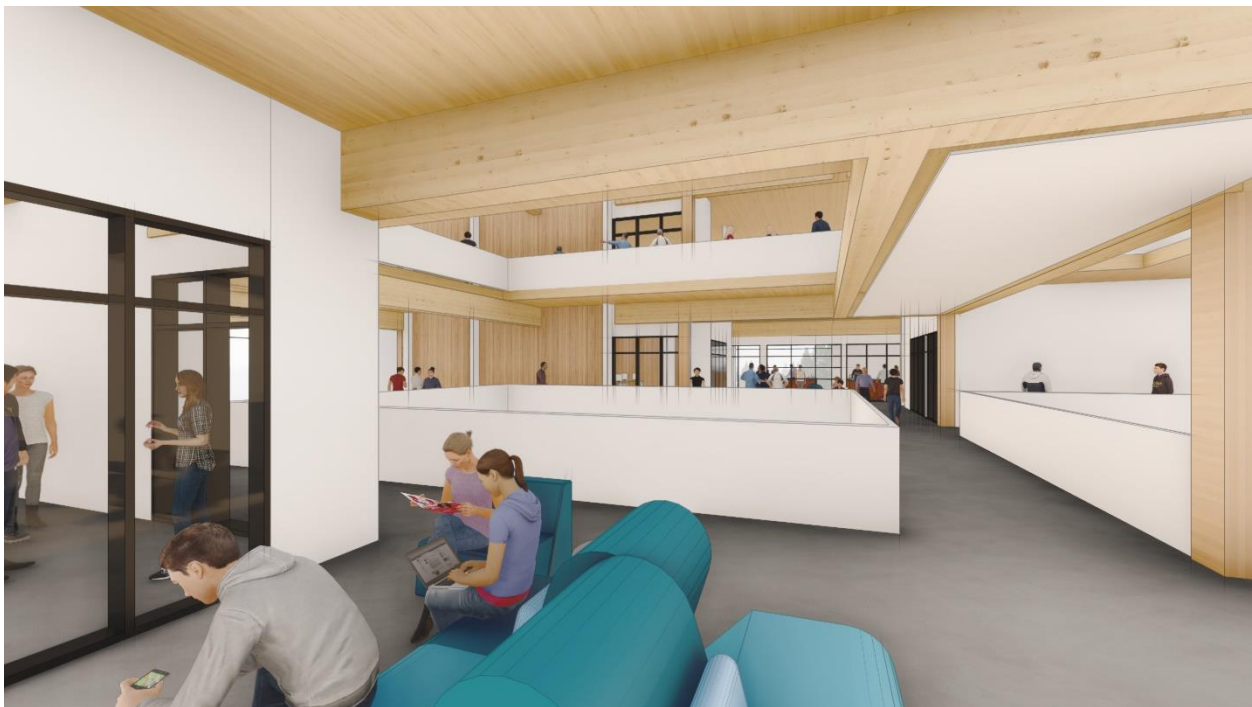
Interior view showing the extent of mass timber construction in a 4 storey school
