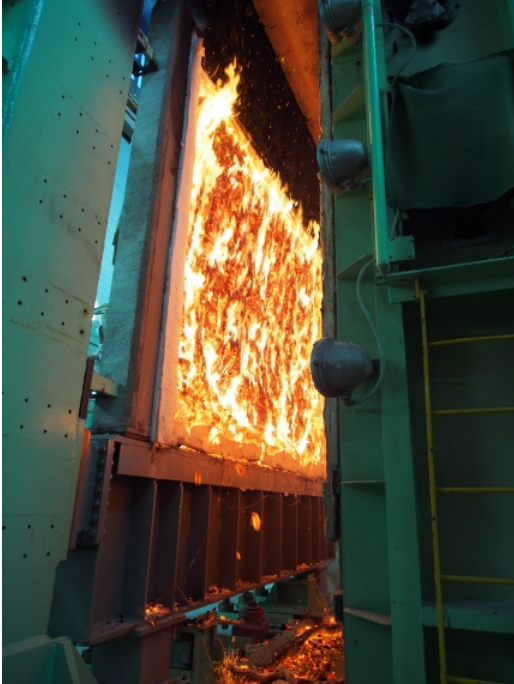
Figure 30. 2x8 NLT wall after test.
