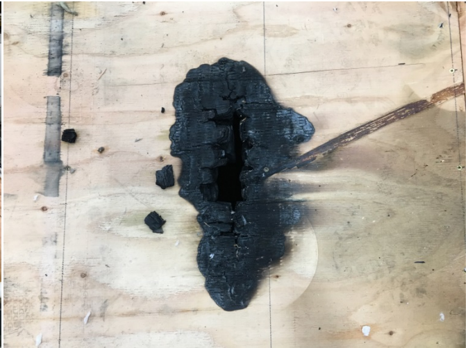
Figure 46. 2x6 NLT floor location of burn-through.
