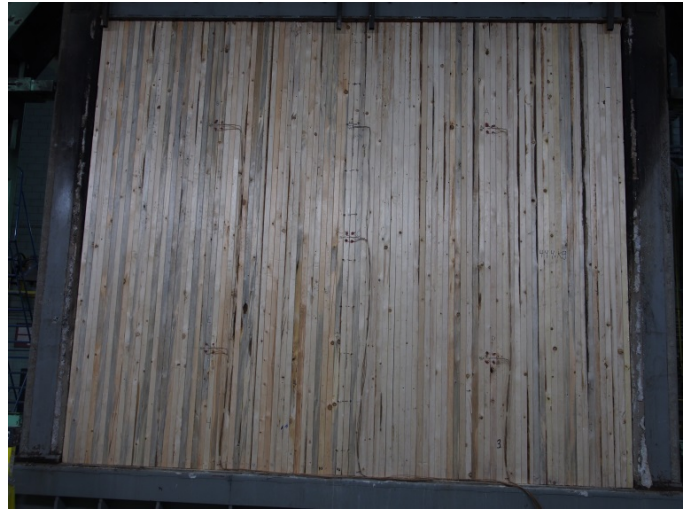
Figure 8. 2x8 NLT wall unexposed side before gypsum application.
