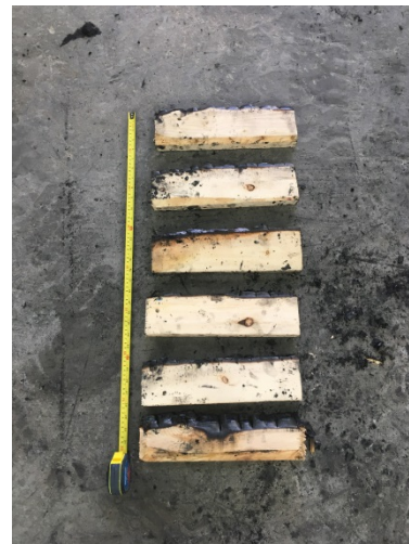
Figure 29. 2x6 NLT wall typical depth of char.
