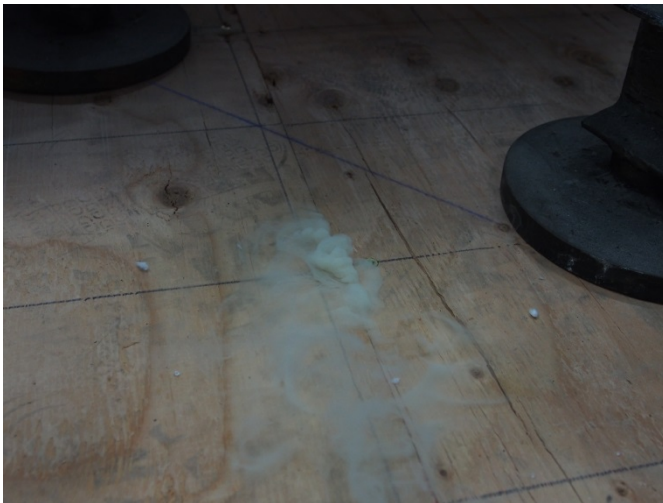
Figure 39. 2x6 NLT floor intermittent light smoke leakage during test.
