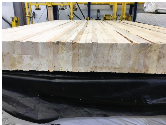
Figure 52. Cross-section of NLT.
