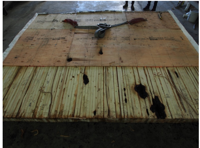
Figure 27. 2x6 NLT wall unexposed surface after plywood removal.
