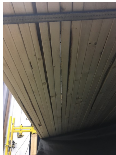
Figure 50. Light able to pass through assembly.
