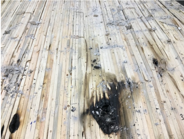
Figure 36. 2x8 NLT wall unexposed surface after test, gypsum removed.
