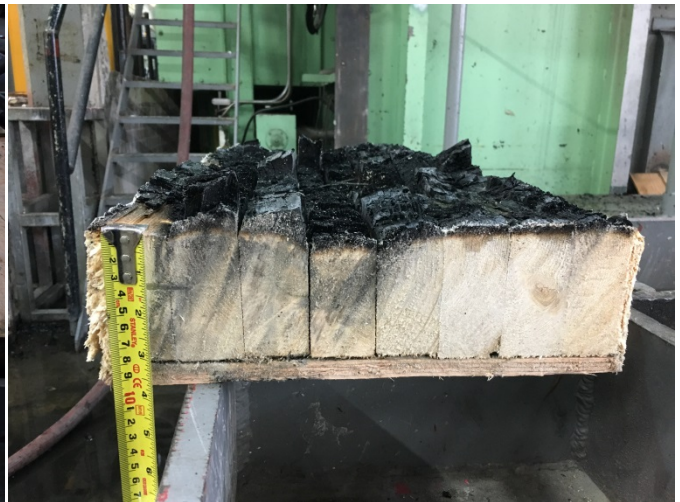
Figure 48. 2x6 NLT floor depth of char in cut sample.
