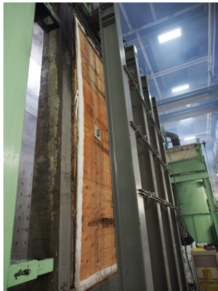
Figure 22. 2x6 NLT wall structural failure, deflection.
