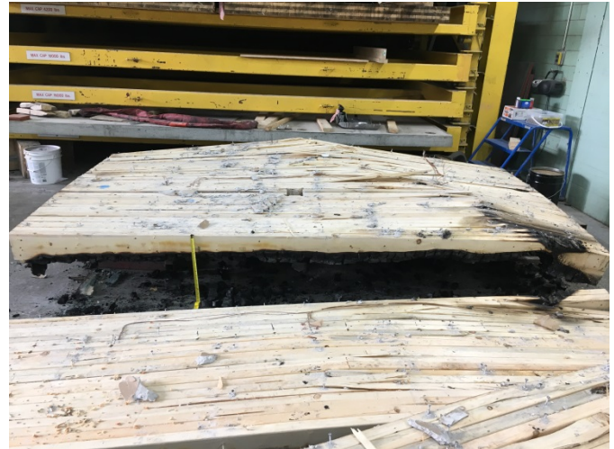
Figure 37. 2x8 NLT wall depth of charring along length of board.
