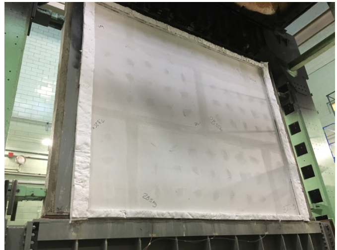
Figure 12. 2x8 NLT exposed side before test.
