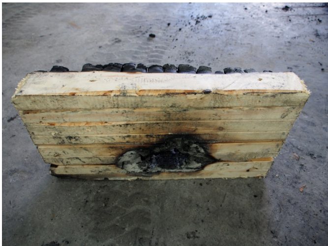
Figure 28. 2x6 NLT wall section taken at primary failure.
