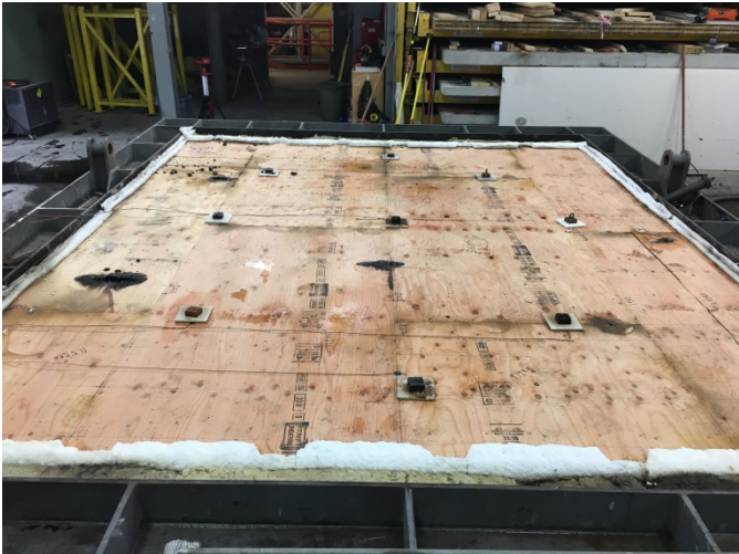
Figure 45. 2x6 NLT floor unexposed surface after test. Charring through plywood after end of test.
