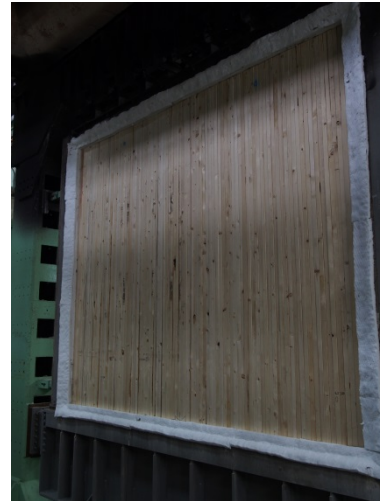
Figure 3. 2x6 NLT Exposed side of assembly.
