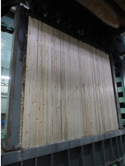
Figure 7. 2x8 NLT wall exposed side before gypsum application.
