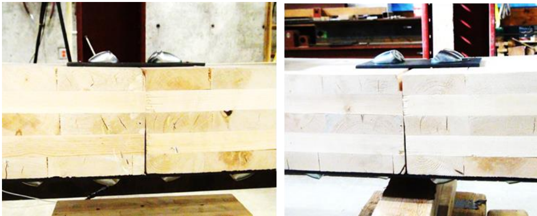
Figure 13 Deformation at the joint under bending
