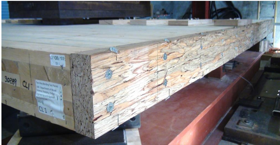
Figure 9 Rim beam attached to the edge of the joined panel
