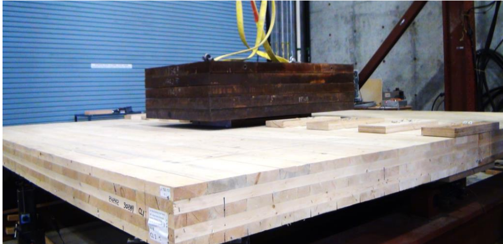
Figure 8 Loading of the joined panel
