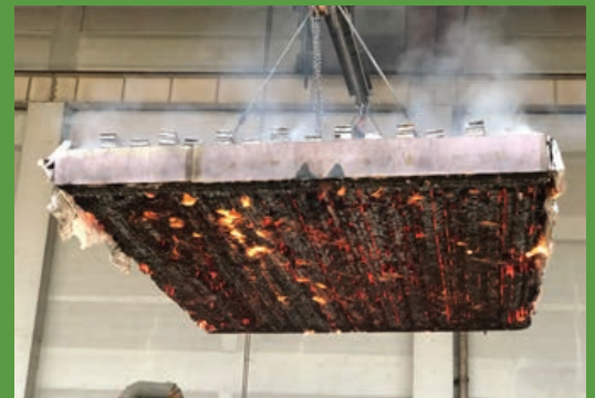
NLT Fire Resistance Test, Beijing | Photo: Canada Wood China
